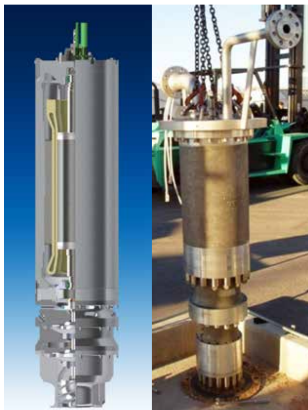
Figure 3. Cargo pump (left) and line packing pump (right).
